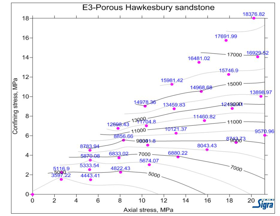
Poisson's ratio  $V_{13}$
