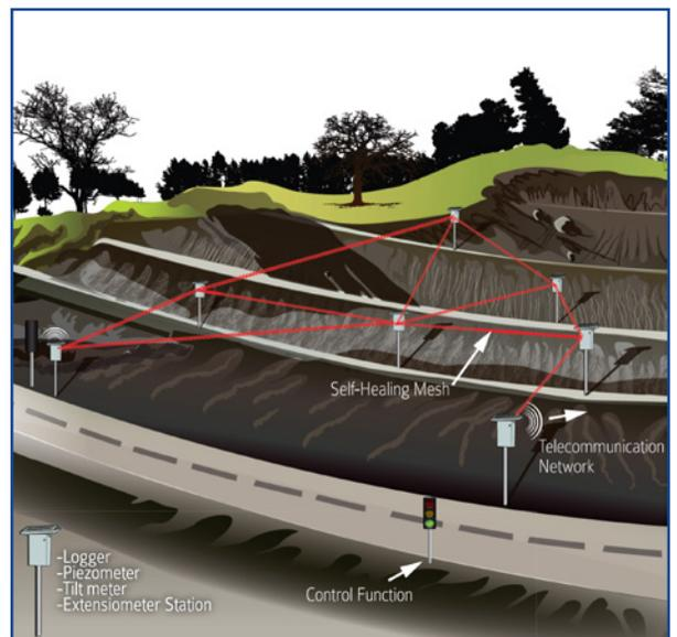
*Landslide monitoring and warning system*
