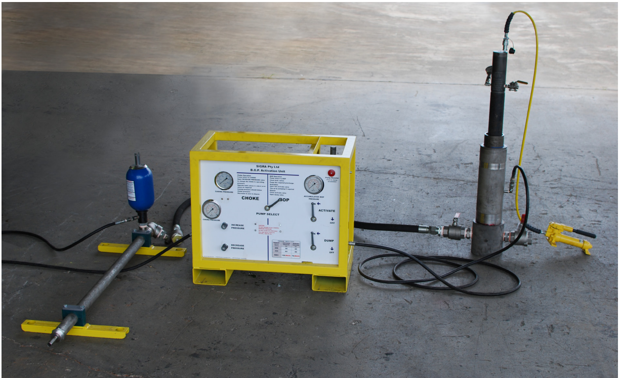
Choke, activation unit and BOP with wire line stripper attached Shown for clarity without low profile mud bucket.
