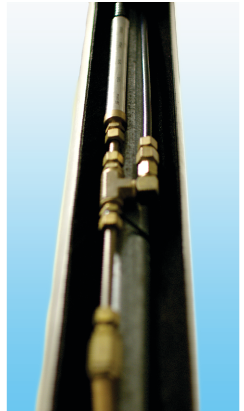
Sigra 5MPa vibrating wire transducer paired with Sigra's cement displacement technology
