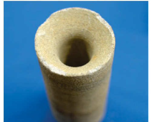
Core sample with countersink and pilot
