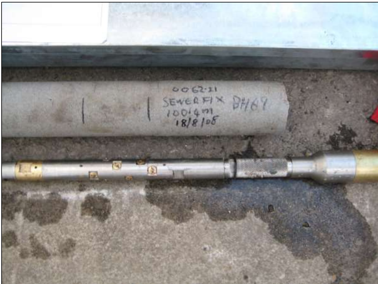
Figure 3. IST2D overcore tool and overcore from which it has just been extracted.
