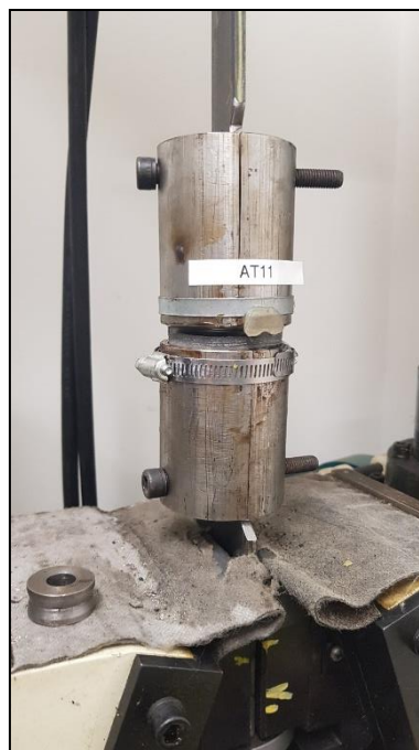
Figure 29: Example of Axial Tensile Test
