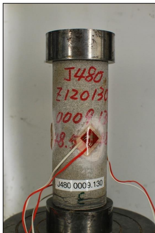
Figure 2: Uniaxial test specimen fitted with axial and circumferential strain rosettes
