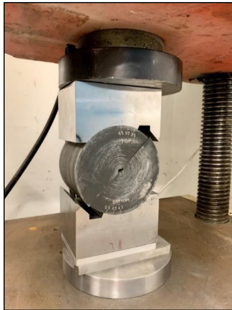
Figure 16: Modified GOST Shear Test Setup
