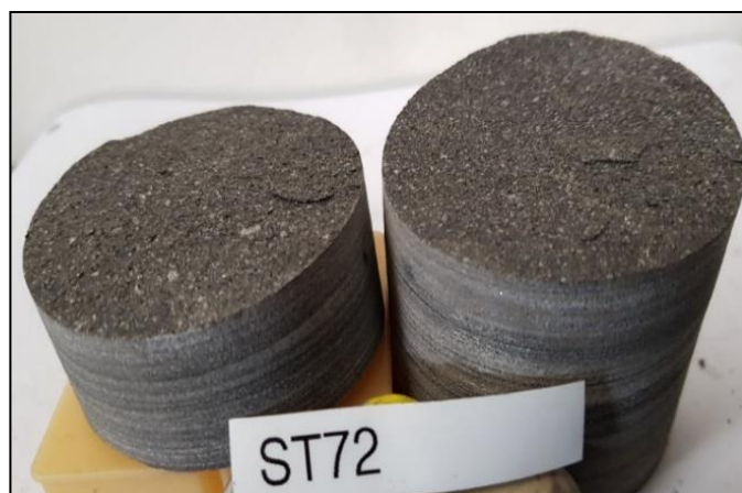
Figure 14: Test sample after failure, Side View
