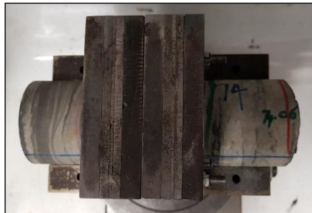
Figure 13: Core Shear Strength Testing Apparatus, Top view
