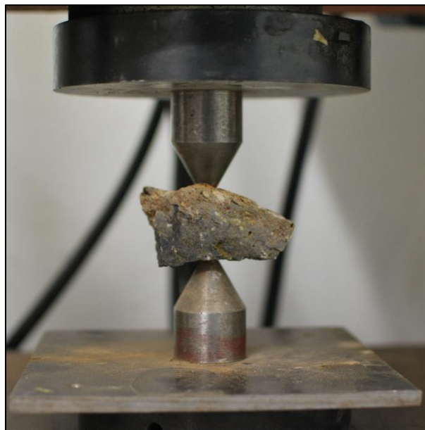
Figure 32: Point load test of an irregular specimen in the laboratory.
