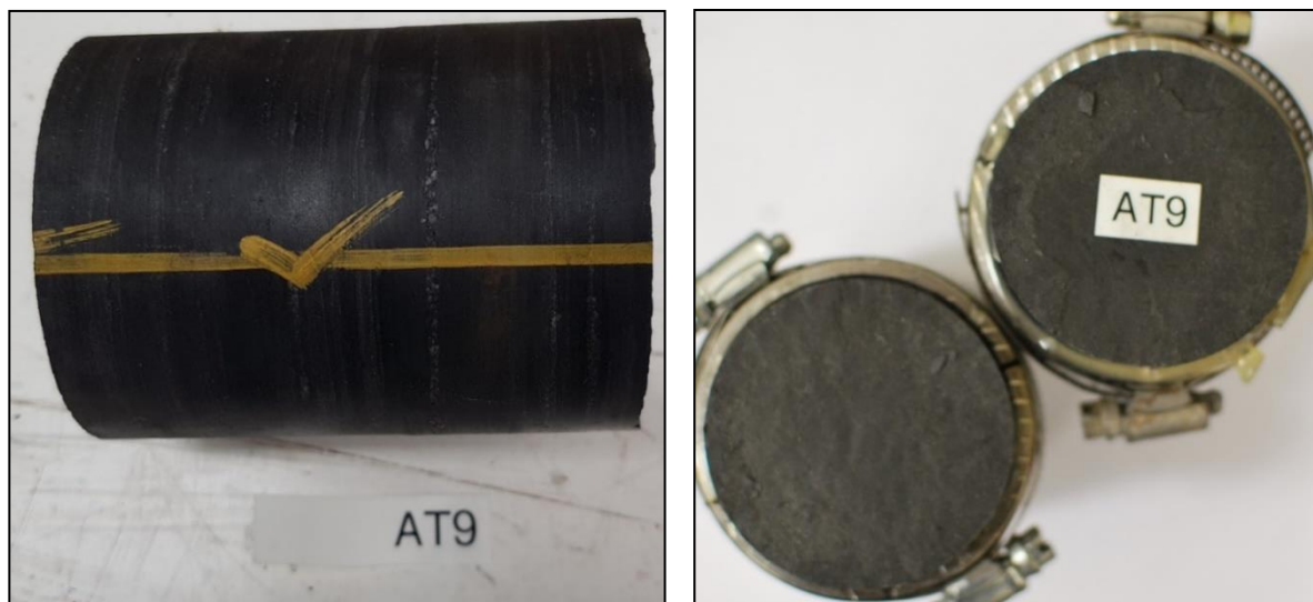
Figure 30: Tensile test specimen before and after testing.
