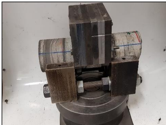
Figure 12: Direct shear test on a core specimen
