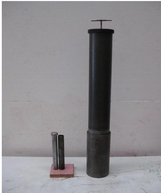
Figure 35: Drop hammer equipment – measuring cylinder with scale and tube with drop hammer.
