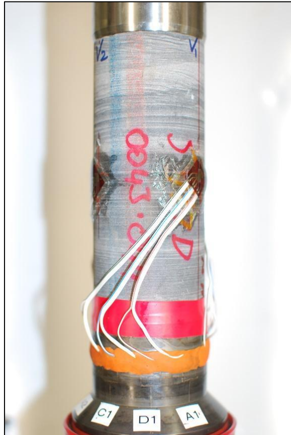
Figure 20: Showing a fine grained silty sandstone core fitted with strain gauge rosettes within the triaxial cell prior to the sleeve being fitted.
