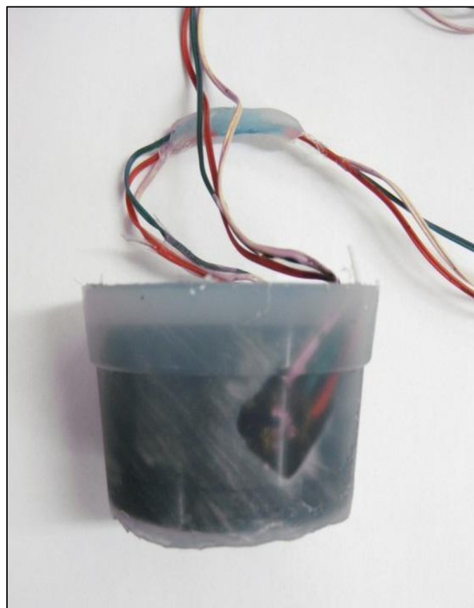
Figure 23: Strain gauged phyllite sample cast in silicone resin.
