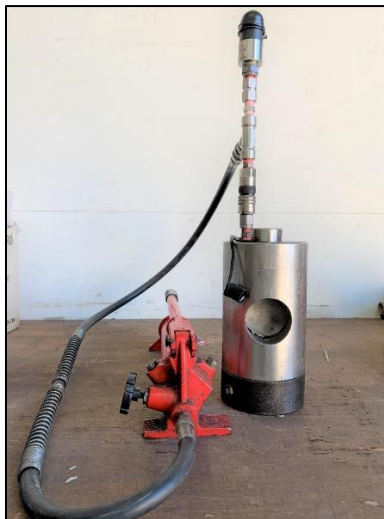
Figure 33: Site Brazilian test equipment – test cylinder with pressure pump
