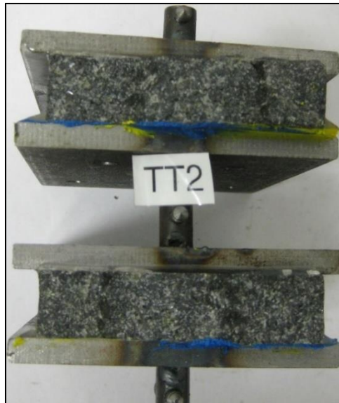
Figure 27: Failed transverse tensile test disc.
