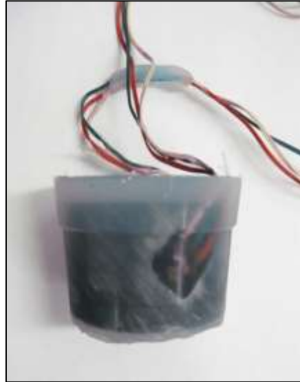
Figure 3. A hydrostatic sample fitted with rosettes and cast in silicone resin. Note the bedding of the phyllite sample which is at an angle to the core.
