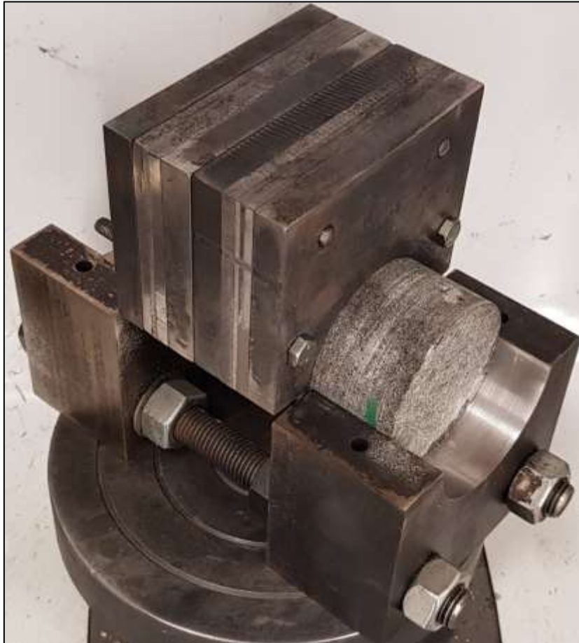
Figure 4. Direct shear test on a core specimen.
