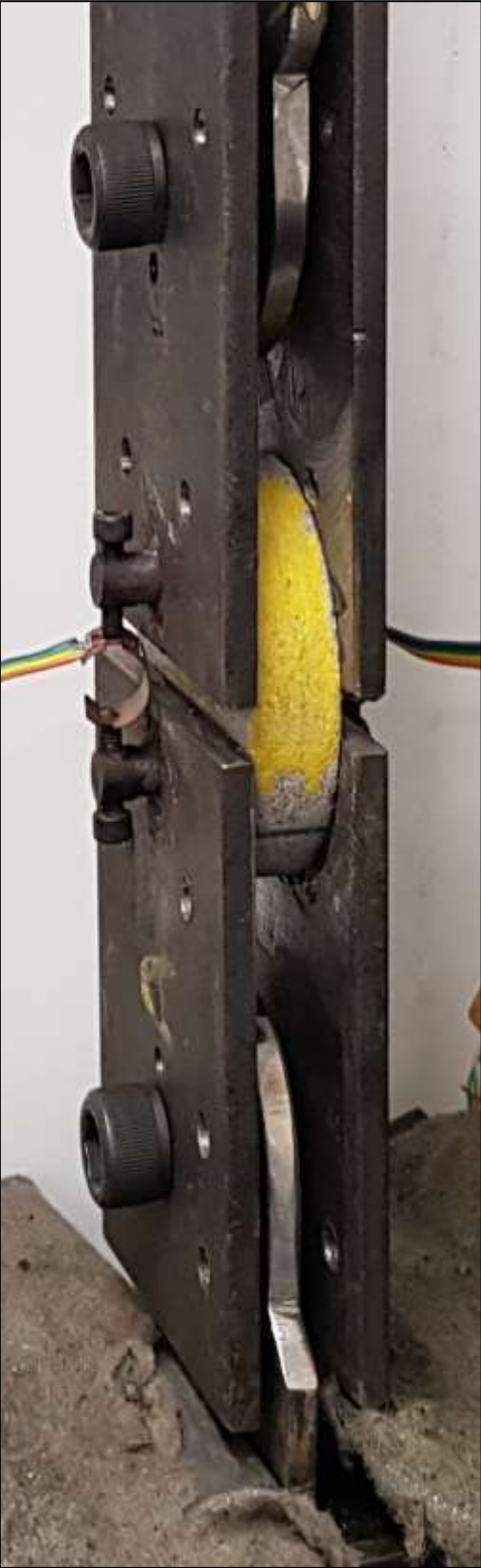
Figure 5. Transverse tensile rock test setup.
