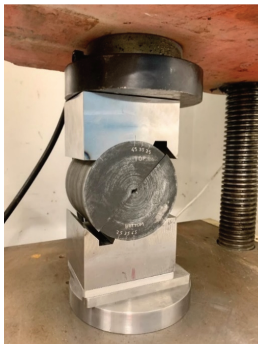
Figure 16 Modified GOST shear test setup in universal test machine
