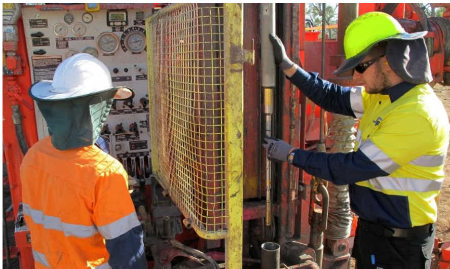
Figure 1: Sigra IST stress measurement tool in use in HQ wireline coring
