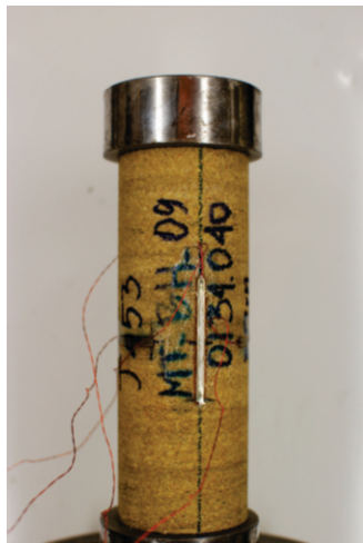
Core sample prepared for testing in the laboratory
