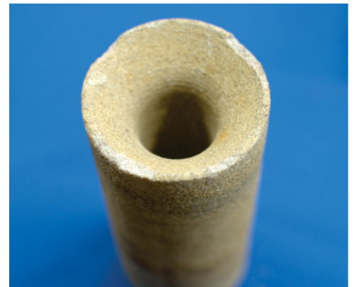
Core sample with countersink and pilot
