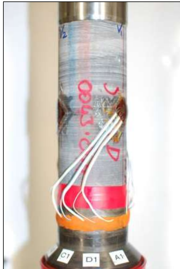
Figure 1. Showing a fine grained silty sandstone core fitted with strain gauge rosettes within the triaxial cell prior to the sleeve being fitted
