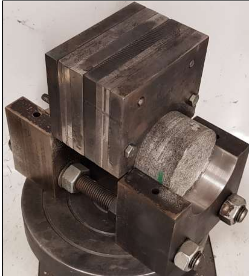
Figure 4. Direct shear test on a core specimen.
