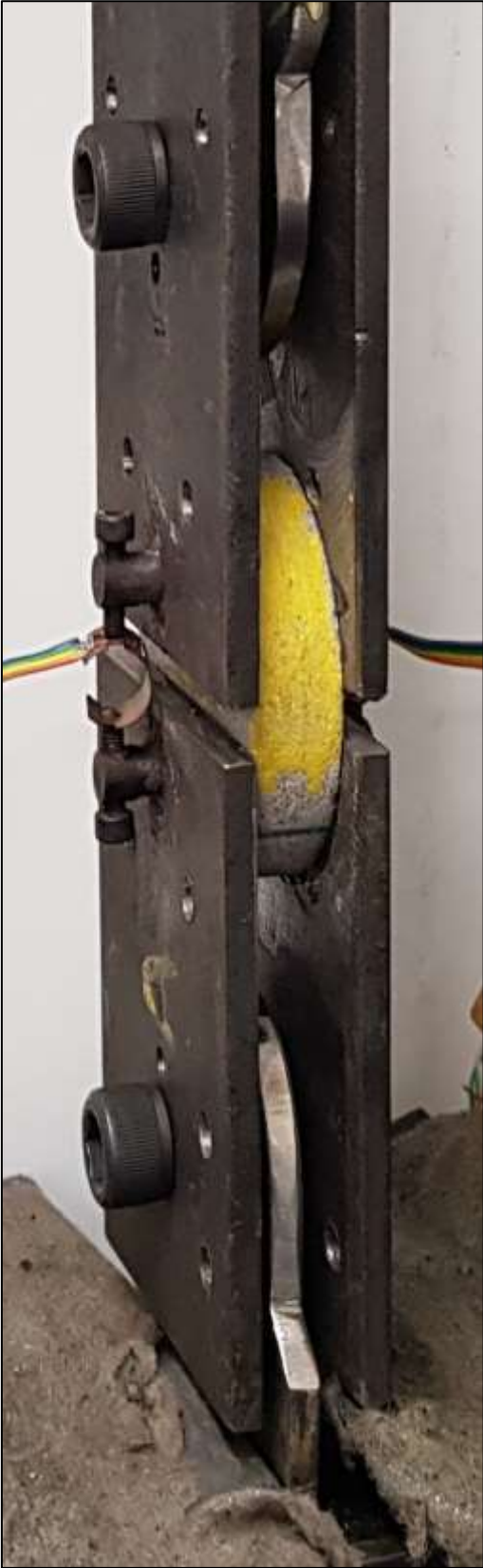
Figure 5. Transverse tensile rock test setup.
