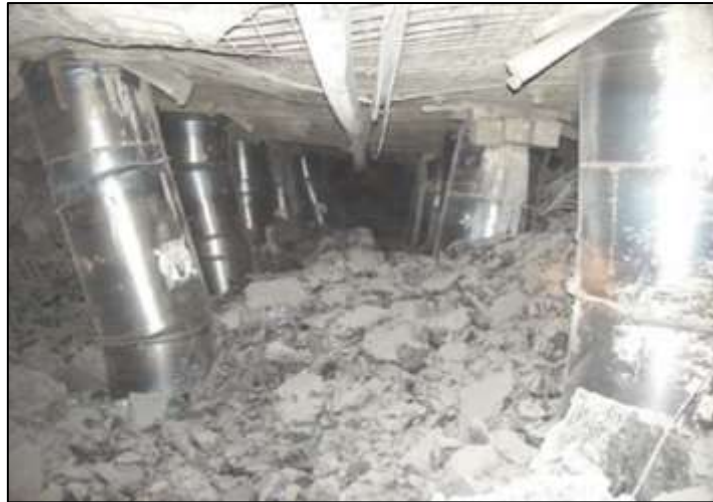
Figure 16. Elk Creek longwall tailgate coalburst (Mark 2016)
