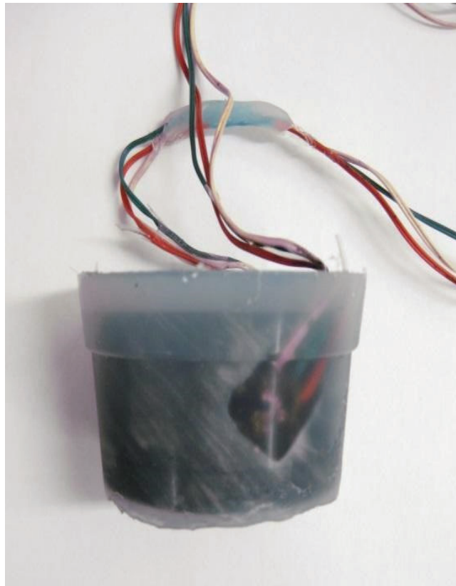
Figure 11 Strain gauged sample of phyllite cast in silicone resin for hydrostatic testing
