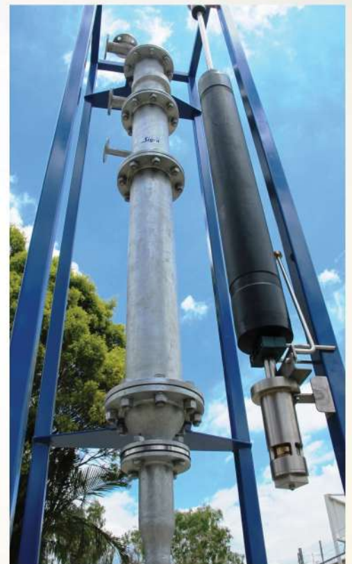
Separator shown on a picture is mounted for exhibition purposes. Float and valve mechanism shown at right
