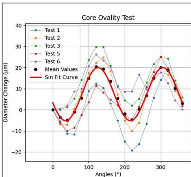
Figure 11. Traces in  $\mu\text{m}$  from core ovality testing.
