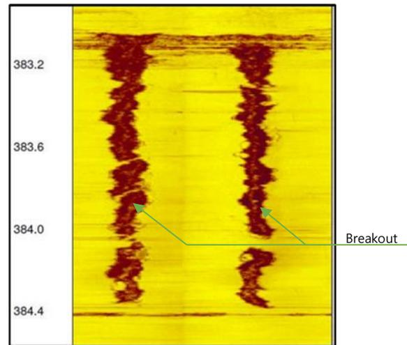
Figure 8. ATV view of breakout in a siltstone.
