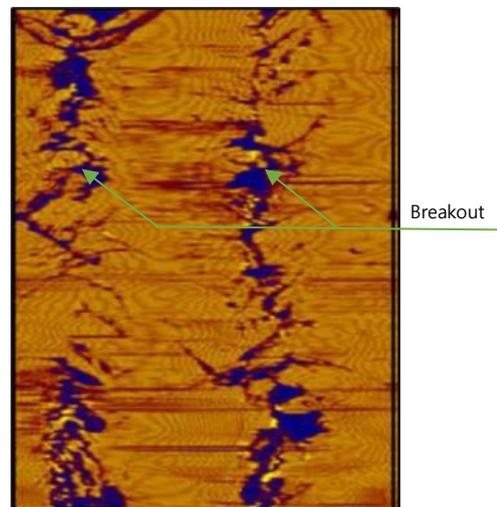
Figure 9. ATV view of breakout in a metasiltstone.
