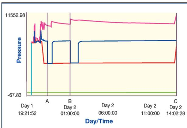
Figure 6. A total test plot of a drill stem test.
