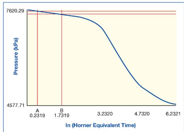
Figure 8. The build-up plot with respect to Horner Equivalent time.
