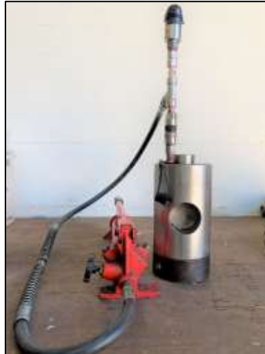
Figure 6: Site Brazilian test equipment – test cylinder with hand operated pump
