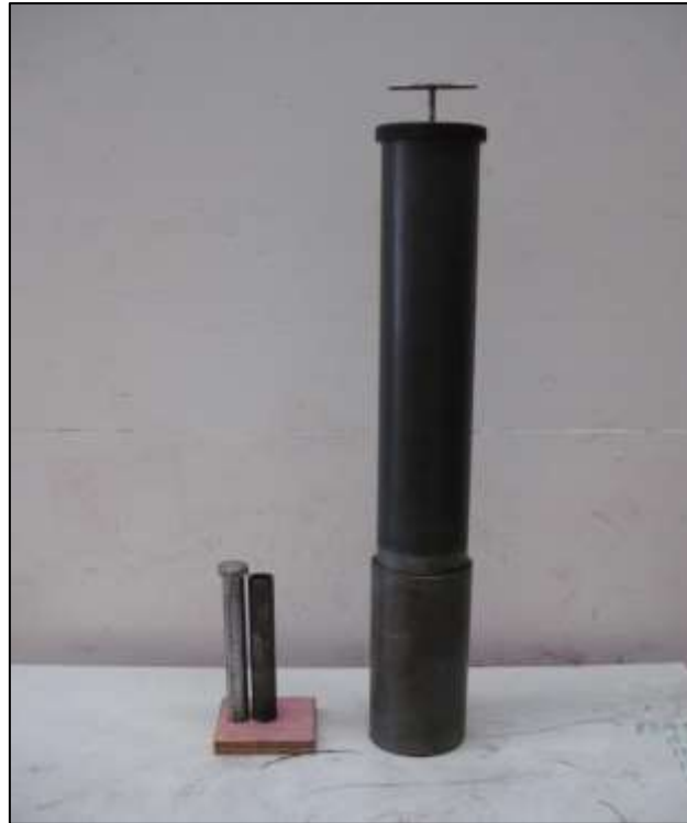
Figure 12. Drop hammer equipment – measuring cylinder with scale and tube with drop hammer.
