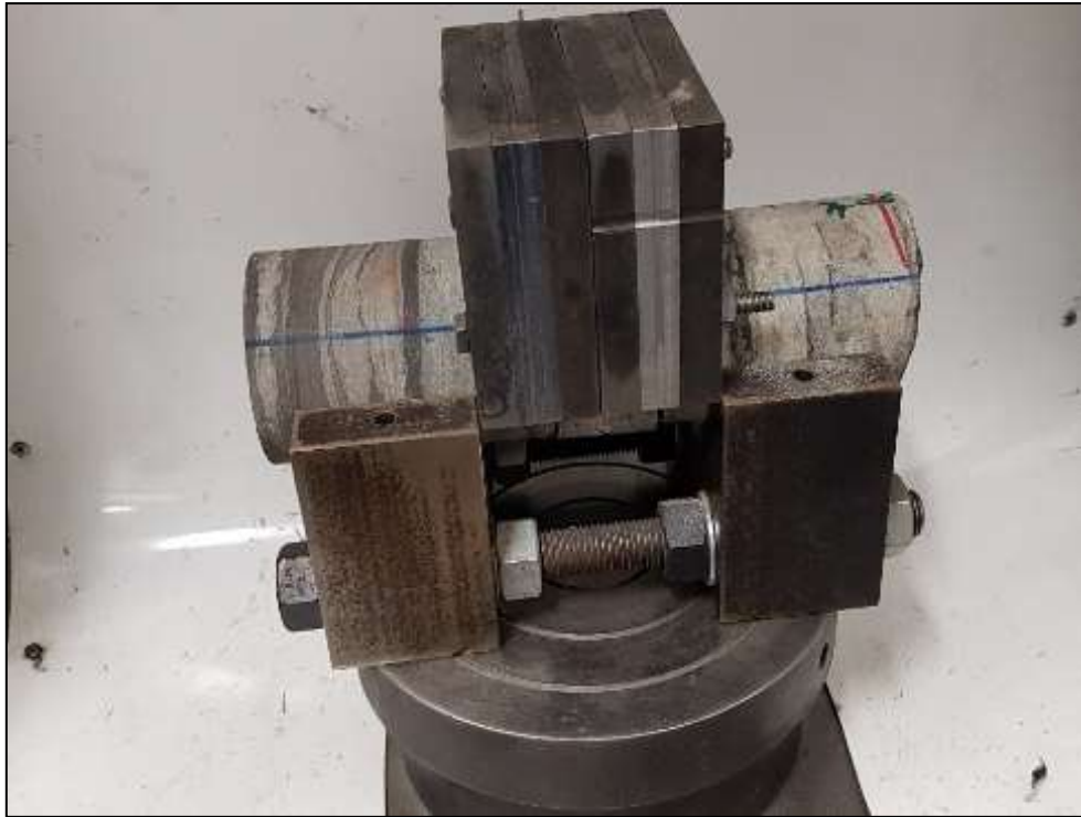
Figure 9. Direct shear test of core.
