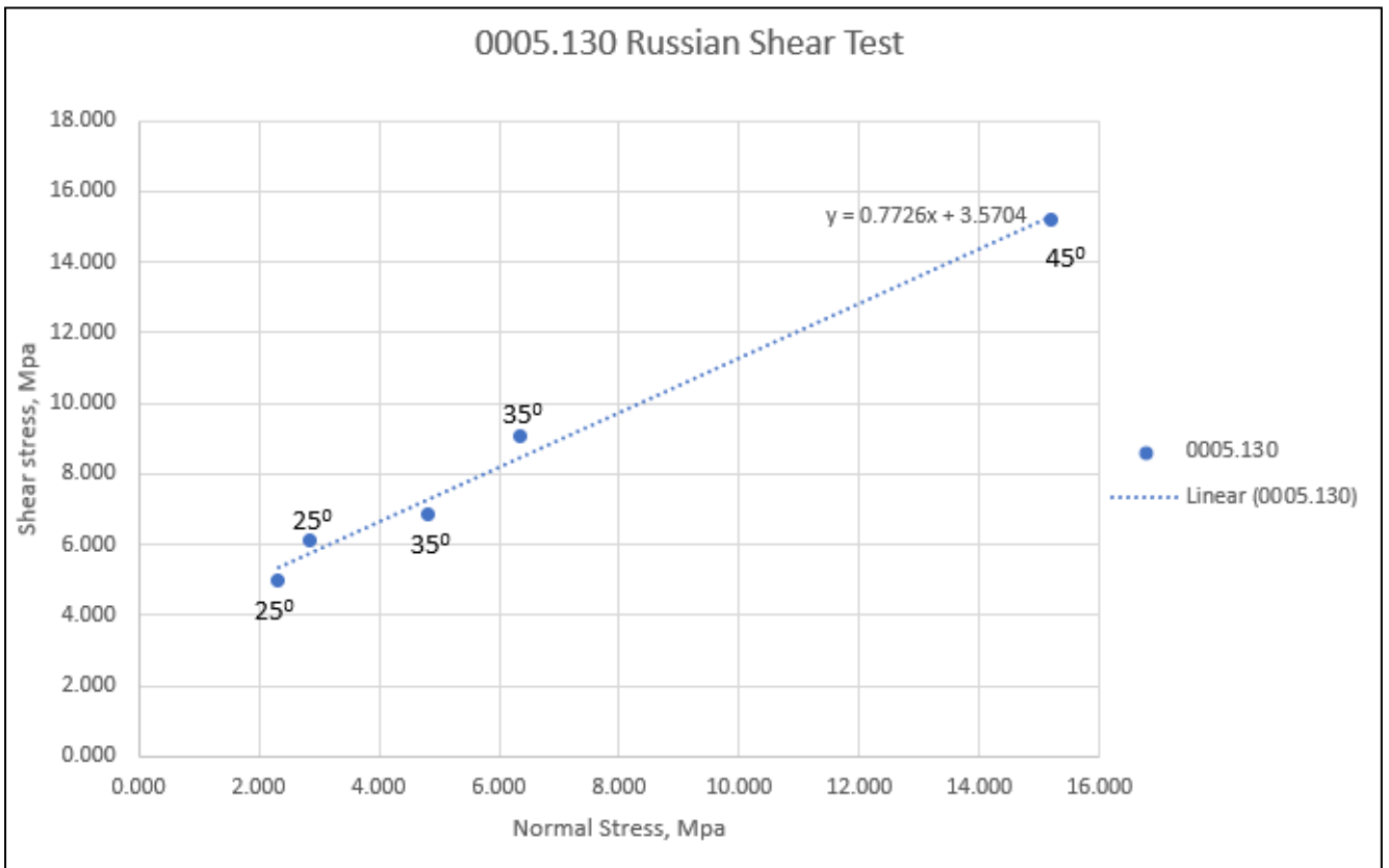
Figure 11. Modified GOST shear test results with fitted Mohr-Coulomb failure envelope.
