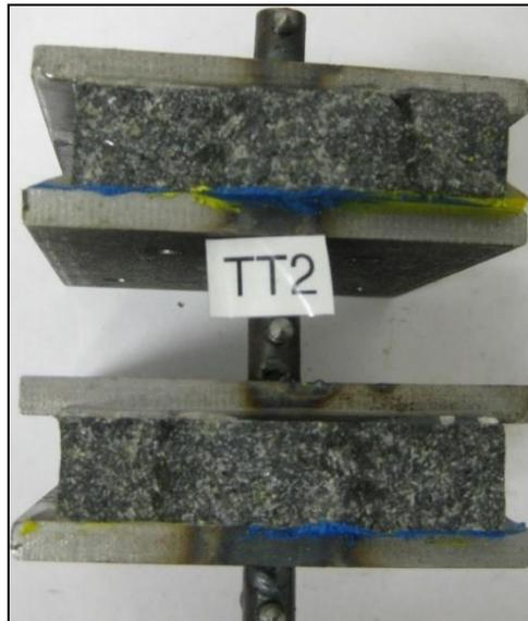
**Figure 27: Failed transverse tensile test disc.**
