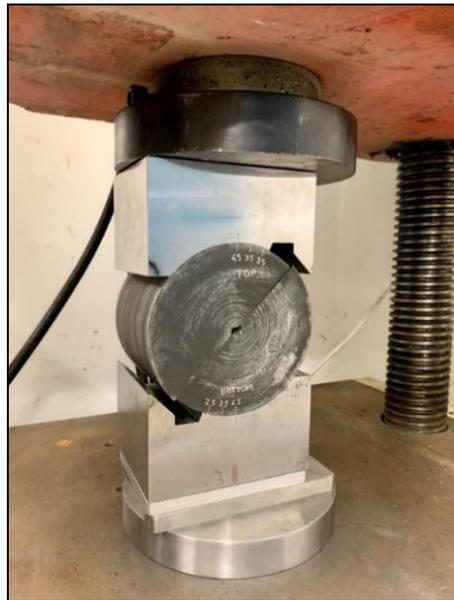
Figure 16: Modified GOST Shear Test Setup
