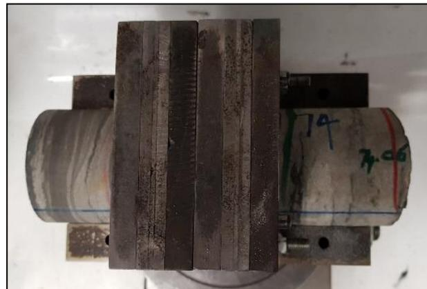
**Figure 13: Core Shear Strength Testing Apparatus, Top view**
