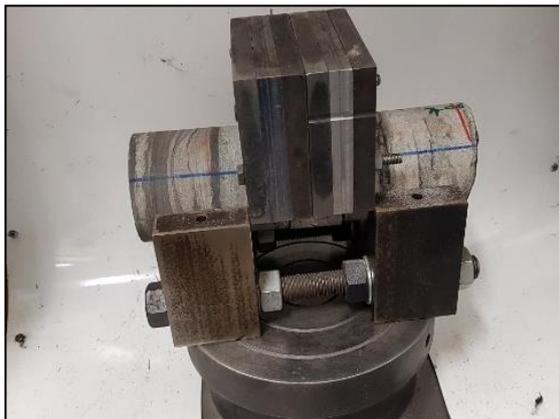
**Figure 12: Direct shear test on a core specimen**
