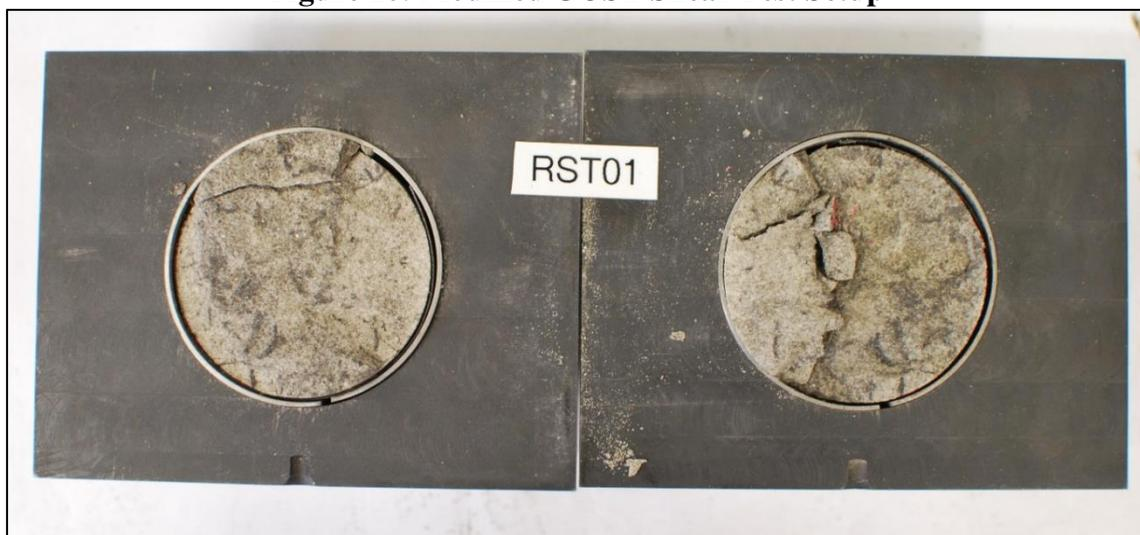
Figure 17: View of failure surface.
